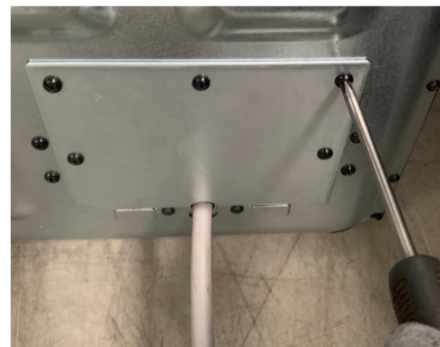
Assemble cover and tighten screws.
